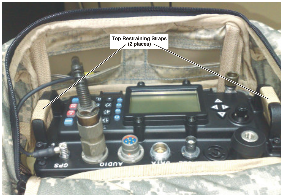
Figure 2-5. Detail of Transceiver in its Carrying Harness
