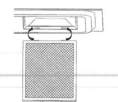
3. To reinstall the exhaust ventilation filter, infix the hooks into the holes of base plate, then pull the lever and toward oven to lock Reinstall the 2nd filter using the same procedure
