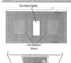
1. To remove the exhaust ventilation filters, pull the lever, then pull filter downward. The filter will drop out. Repeat for the 2nd filter.
