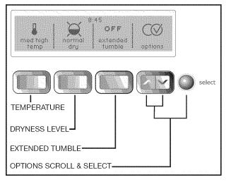
Auto Dry cycles take the guesswork out of selecting the correct drying time for each load. Moisture sensing bars at the back of the dryer drum sense the moisture level of the load as it tumbles through the heated air. With Auto Dry cycles, the load will automatically be dried at the selected temperature to the desired dryness level.
