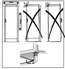
there is good air circulation around the cabinet and that the air channels below and behind the cabinet are not blocked. The ventilation space above the cabinet must be at least 4 cm.
