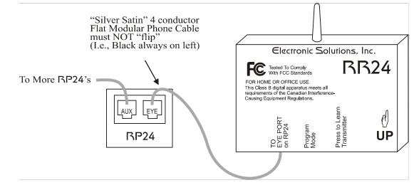
The RR24 unit must connect to an Eye Jack on a RP24 or splitter. If the eye connects to a splitter, then the Main jack next to it **must** connect to the Eye Jack on an RP24.
