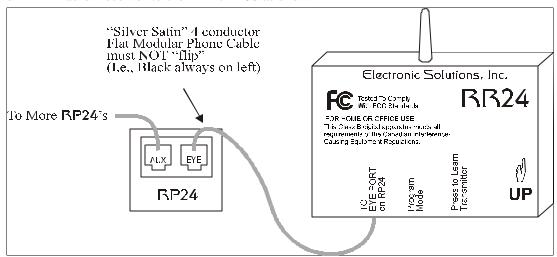
The RR24 unit must connect to an Eye Jack on a RP24/RP60 or splitter. If the eye connects to a splitter, then the Main jack next to it **must** connect to the Eye Jack on an RP24/RP60.
