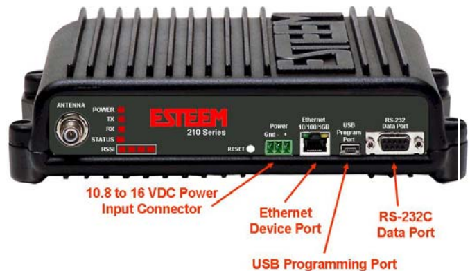
Figure 4: 195C/M Front Panel Overview
