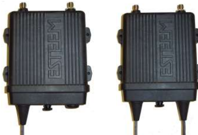
Figure 9: Face Plate Cover Installed on ESTeem
