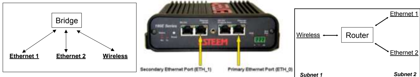
Figure 5: Bridge and Router Configuration for Ethernet Ports
