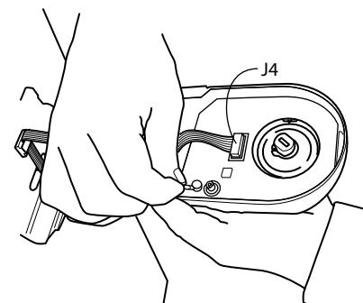
Attach other connector to the port on the green circuit board just below the top left screw. CONNECT ANTENNA is labeled (see picture ).
