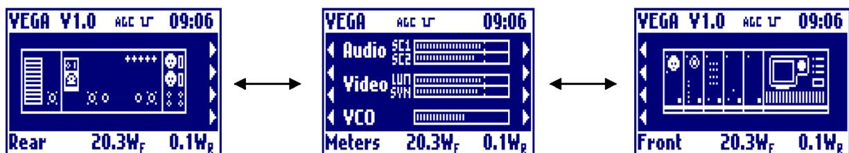
To enter the menu of the individual modules, select the module from the menu with the graphical image of VEGA, both the rear and the front view. After clicking, a blinking arc will show in what module you can enter clicking on the knob. To change module, rotate the knob.
