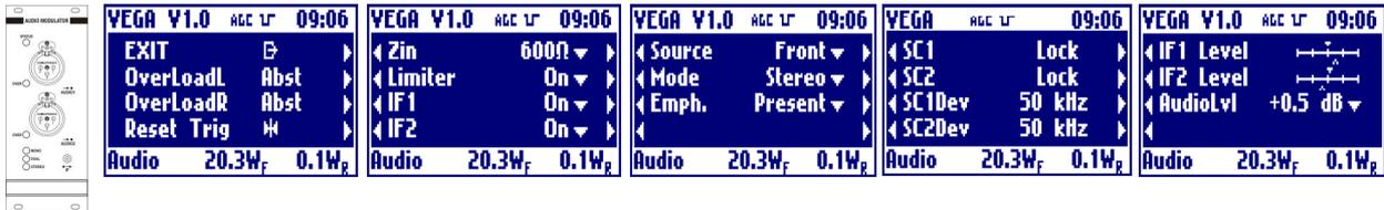
The last menu is showed as in stereo or mono mode settings. If the mode is set for a dual sound audio modulation the last menu become the one below, because you can select to adjust the audio level to different values.
