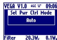
*ATTENTION: for safety operation is better to set 0% to the power level that in not selected. For example is AUTO power control mode is selected, is better to set 0% to the Power Level in manual mode. In this way, after a change, the power will start from 0W.*
