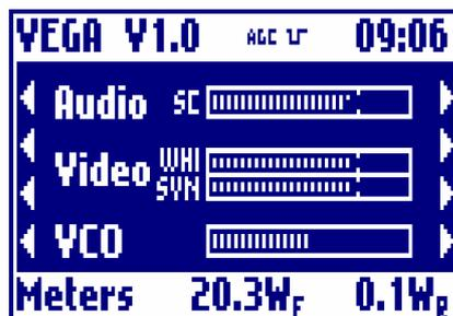
All of the menus of the VEGA contain a top bar which shows the name of the apparatus, the firmware version of the display board and the current time, and a bottom bar showing the reading of the output forward and reflected power and a summary of the current menu.
