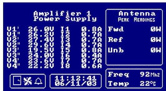
Note that no numerical value is shown for amplifiers which are not communicating with the control module.
