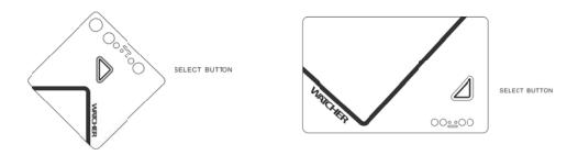
The pendant and card each have one button that is used to pair up with Watcher. Once the RF is enabled on Watcher, scroll down on the menu and select the pair-up option, and press the select button on the pendant/card to connect to your Watcher immediately.
