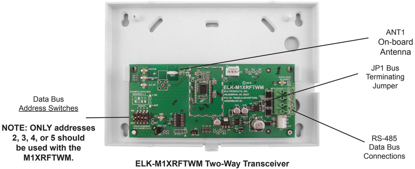
NOTE: Jumper JP1 makes it convenient to terminate the RS-485 Data Bus if this is the last installed device.
