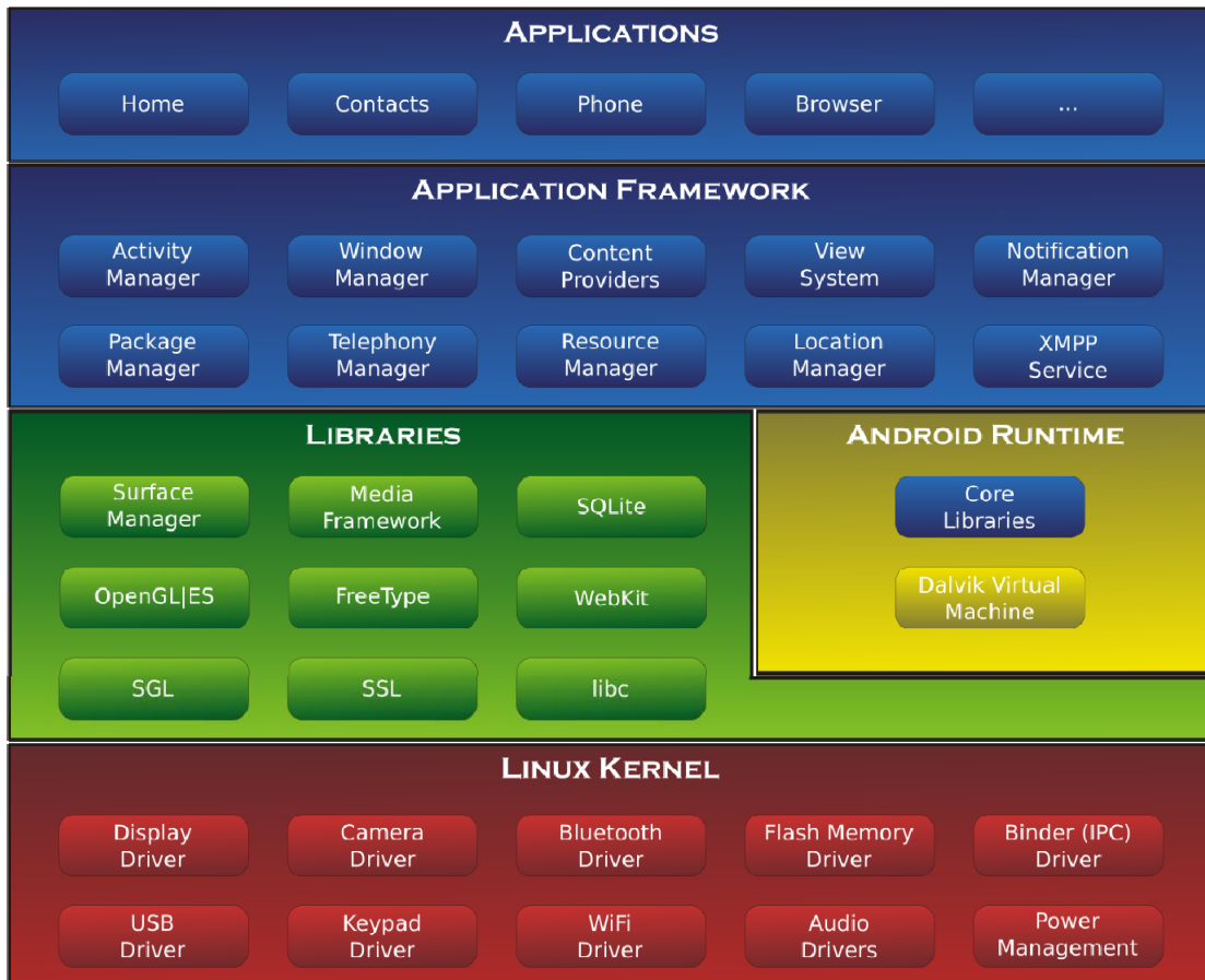
Fig 2-1. Android System Structure
