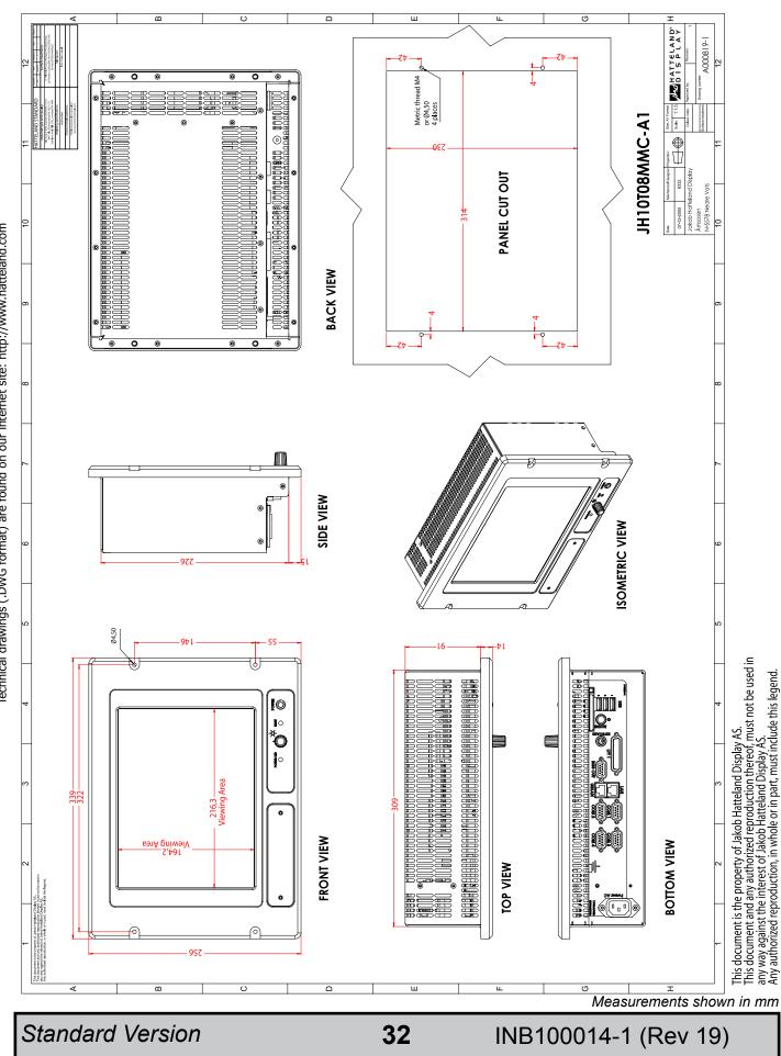
Due to dimensions without decimals, the tolerance on drawings is +/- 1mm (For accurate measurements, measure in AutoCAD) Technical drawings (.DWG format) are found on our internet site: http://www.hatteland.com
