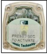
To Activate the sensor from sleep mode, remove the Activation Label. Then press the sensor's call button for at least 7 seconds.
