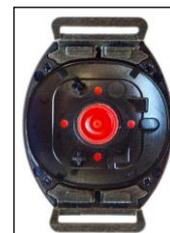
Close the back cover such that the screw holes are correctly aligned. Tighten the 4 screws snugly into place. Do not over-tighten as this may strip the case threads.
