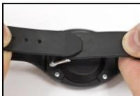
Touch the two ends of the tamper wrist band together.
