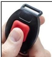
Orient the tag front-cover side up. Next press & hold down the call button for at least 5 seconds.
