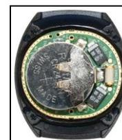
Replace the battery ensuring that the positive (+) side of the battery faces up.
