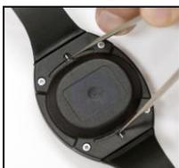
Place the bracelet back cover side up. Using the tips of a metal tweezers, touch the two metal contacts simultaneously.
