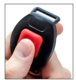
Orient the tag front-cover side up. Next press & hold down the call button for at least 5 seconds.
