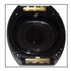
Close the back cover such that the screw holes are correctly aligned. Tighten the 4 screws snugly into place. Do not overtighten as this may strip the case threads
