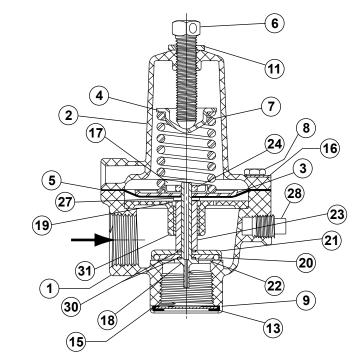
Figure 9. Types 289HH and 1 NPT 289H Relief Valves
