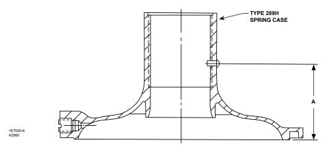
Figure 5. Location of Travel Stop Drive Screw for 2 NPT Type 289H Relief Valve
