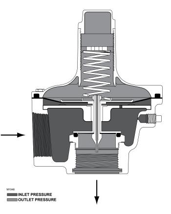
Figure 2. 2 NPT Type 289H Operational Schematic
