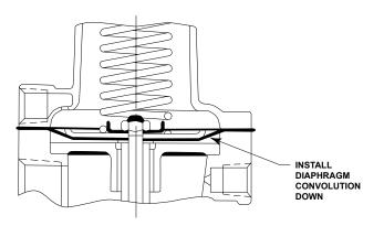
Figure 3. Installation of Diaphragm
