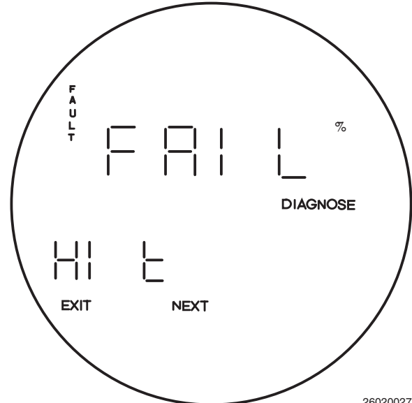
Figure 6-8. Fault 4, High Probe Temperature
