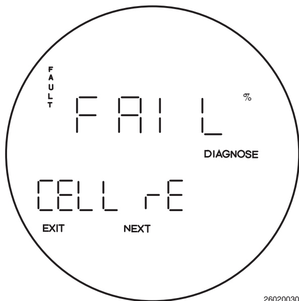
Figure 6-11. Fault 7, Reversed O 2 Cell
