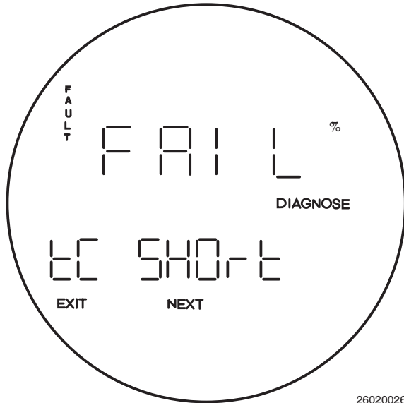
Figure 6-7. Fault 3, Shorted Thermocouple
