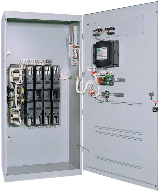
Fig. 2: Four pole, Closed Transition Transfer Switch rated 1000 Amperes in Type 1 enclosure.
