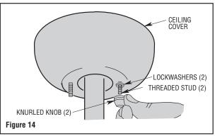
5. Secure the ceiling cover in place by sliding lockwashers over the threaded studs and installing the two knurled knobs (supplied). (Figure 14.) Tighten the knurled knobs securely until the ceiling cover fits snugly against the ceiling and the hole in the ceiling cover is clear of the downrod. Your fan is now wired to be turned on and off from the fan switch.
