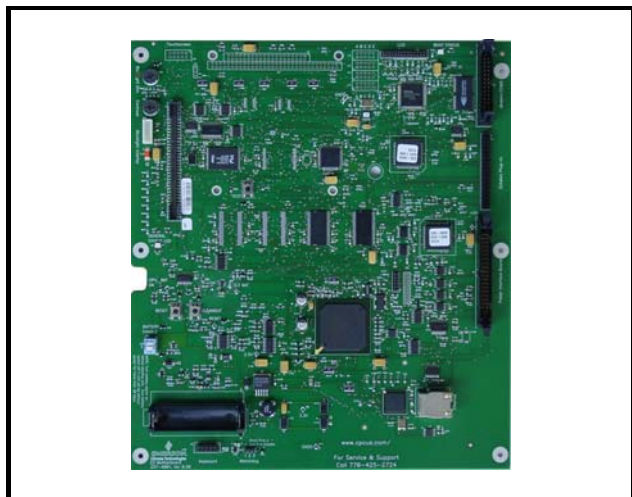
Figure 2-2 - E2 CPU (RX-100 Version Shown)
