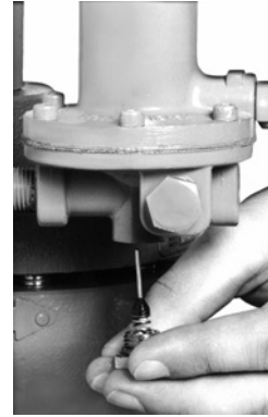
Figure 11. 161EB Series Pilot Trim Removal/Installation
