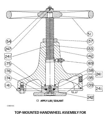
TOP-MOUNTED HANDWHEEL ASSEMBLY FOR SIZE 30, 40, AND 60 ACTUATORS
