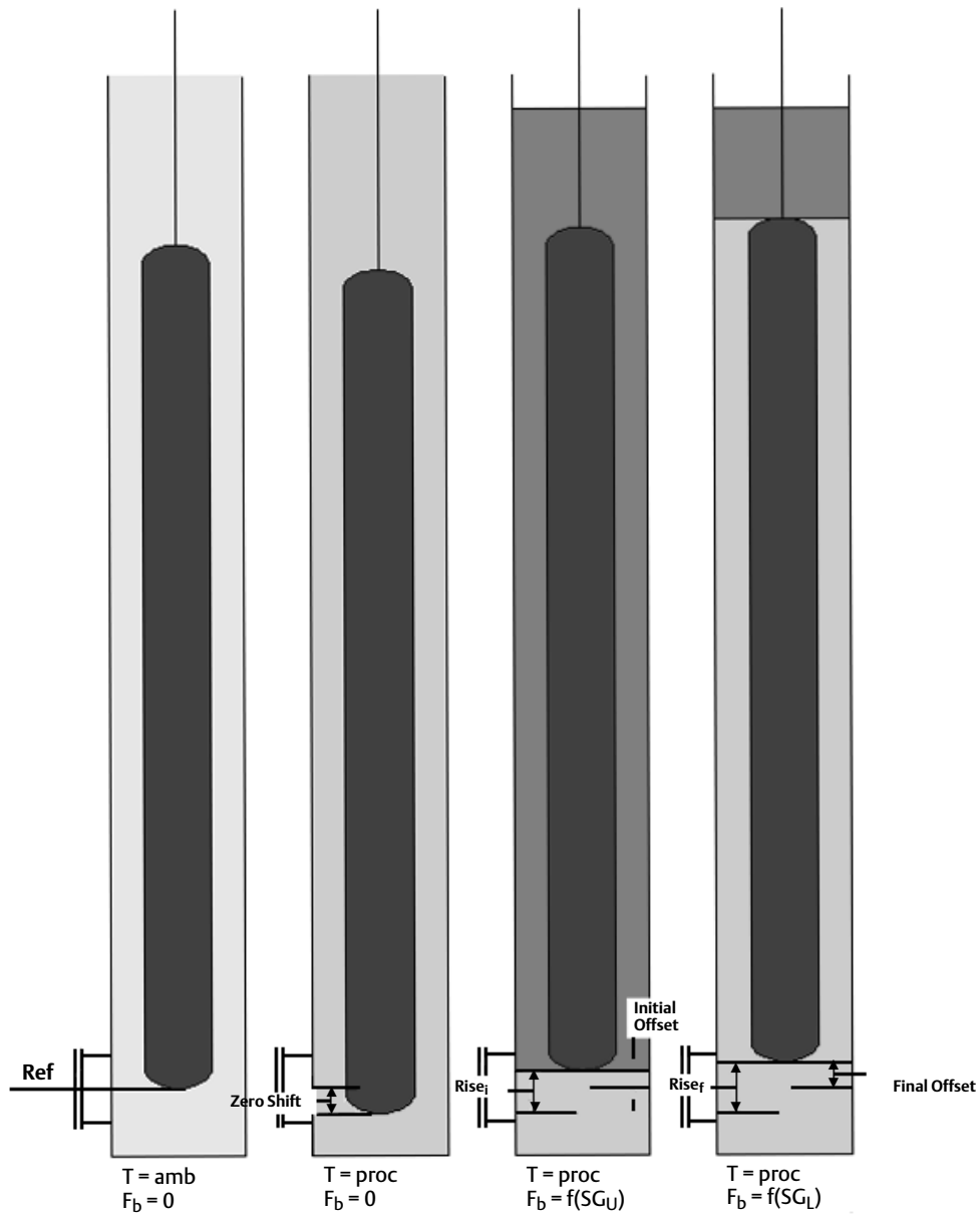
Figure 5. Illustration of Displacer Rise Effect
