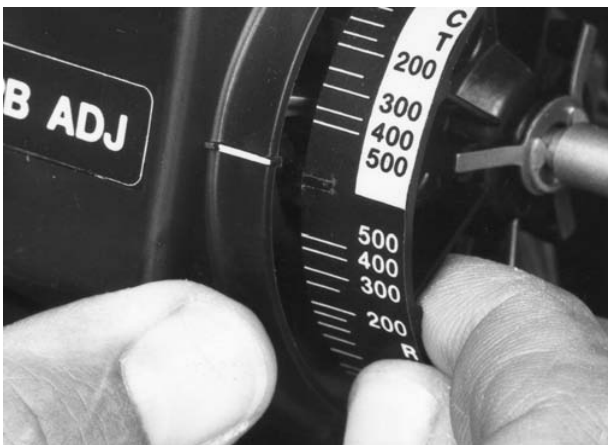
Figure 3-2. Changing Controller Action on Fisher 4195KA Controllers
