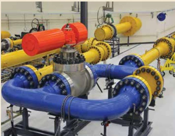
Sizing coefficients for Fisher control valves are based on actual flow tests performed by Emerson engineers. It is not necessary to apply conservative sizing practices; therefore, project costs are reduced.
