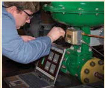
*The cycle life of Fisher control valves is verified. To meet Emerson's pressure swing adsorption quality standard, cycle counts must exceed one million.*
