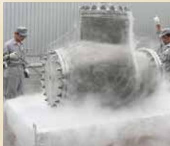
*Whether driven by process temperatures or climate extremes, control valves need to operate as specified. LNG control valves are tested at cryogenic temperatures of -196°C (-321°F).*
