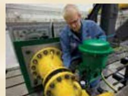
*Fisher control valves are used in safety-critical areas of nuclear power plants and it is imperative that they work when called upon. They undergo rigorous qualification testing to satisfy the requirements of ASME QME-1, IEEE382, IEEE344, and IEEE323.*
