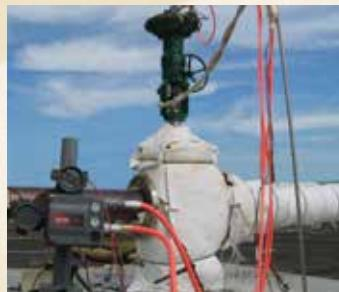
*A refinery valve used in catalytic reforming is tested at 704°C (1300°F). Remote mount solutions for instrumentation decouple the electronics from the process environment for extended temperature range.*
