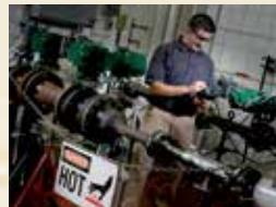
*Testing ensures flexibility of control valve installation orientation. Fisher rotary control valves can be mounted in either horizontal or vertical position without compromising cycle life.*
