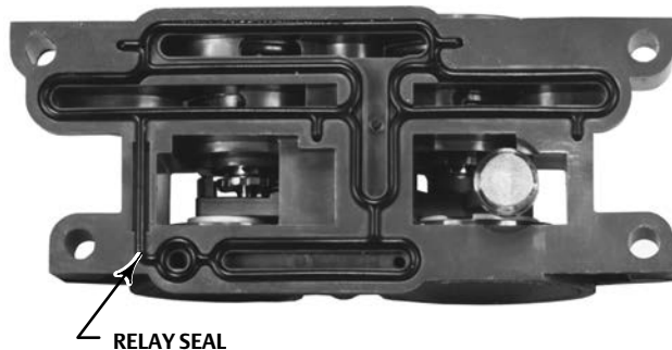
Figure 7-5. Pneumatic Relay Assembly
