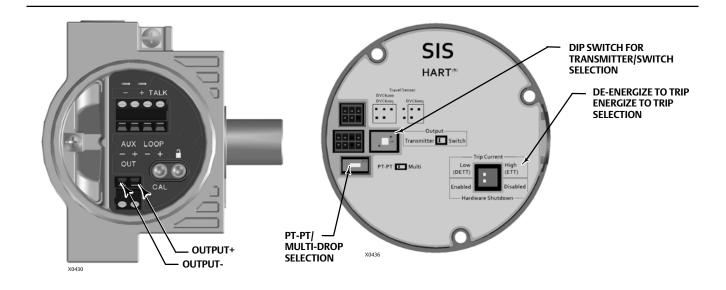
The DVC6200 SIS has an analog shutdown circuit built into the electronics construction. This circuit enables the DVC6200 SIS to perform the safety function through electronics hardware, independent from the device firmware. This function is controlled by two DIP switches:
