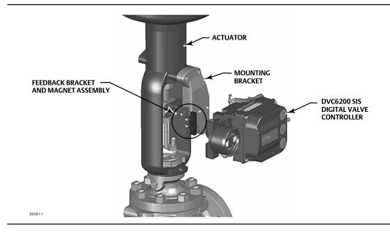
Pneumatic tubing connected to the DVC6200 SIS brings instrument supply air to the DVC6200 SIS and takes controlled output air from the DVC6200 SIS to the actuator. Pressure sensors in the DVC6200 SIS measure these pressure signals and present them as device variables
