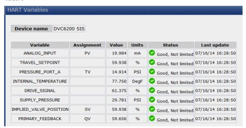
Published Data, used for the Gateway's OPC and Modbus outputs, falls into the following categories:
