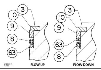
Keys 5\*, 8\*, 9\*, 10\*, and 63\* Fisher EHT Above 450°F (232°C) Using PEEK<sup>(1)</sup> Anti-Extrusion Rings (see figure 22)
