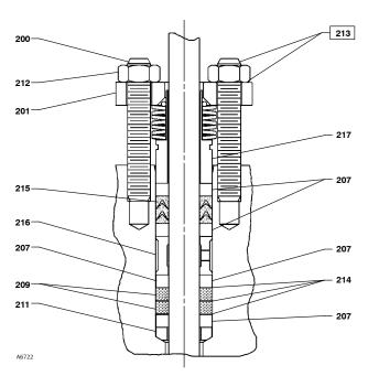
Typical ENVIRO-SEAL Packing System with Duplex Packing
