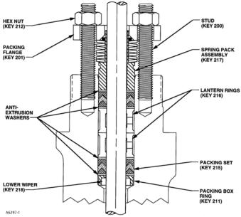
Typical HIGH-SEAL ULF Packing System
