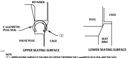
1 UPPER SEATING SURFACE IS THE AREA OF CONTACT BETWEEN THE C-seal METAL PLUG SEAL AND THE CAGE.
