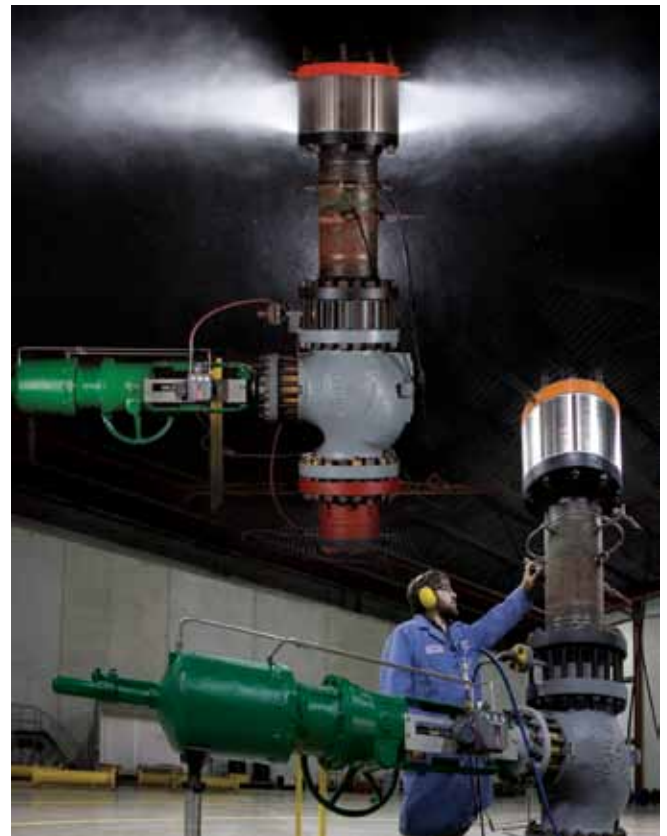
Noise testing of an NPS 12 vent diffuser.
