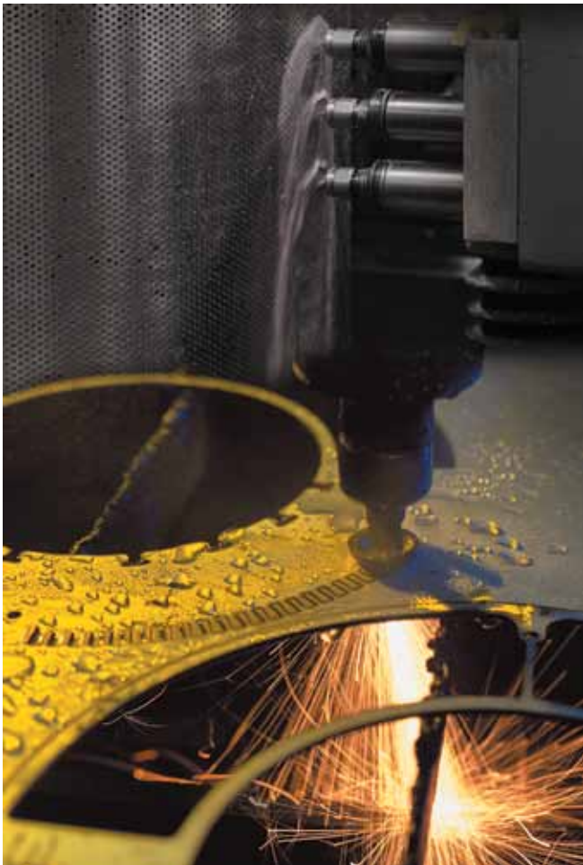
Advanced manufacturing techniques lead to consistent quality and reduced lead-times. Laser cut disks produce tight tolerances consistently for stacked-disk cages. The twelve spindle, high-speed drilling machine reduces the manufacturing time for drilled-hole cages such as Fisher Whisper Trim III.
