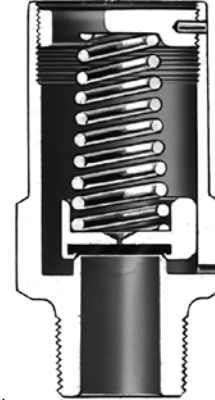
Figure 2. Sectional View of H200 Series Relief Valve
