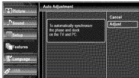
The horizontal/vertical position, clock and phase of the PC screen are automatically adjusted.
