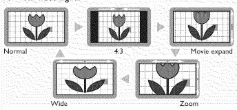
Normal displays a 16:9 picture at its original size.
