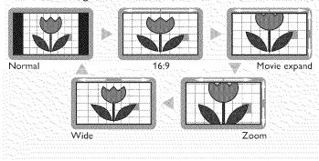
**Normal** displays a 4:3 picture at its original size. Sidebars appear on both edges of the screen.
