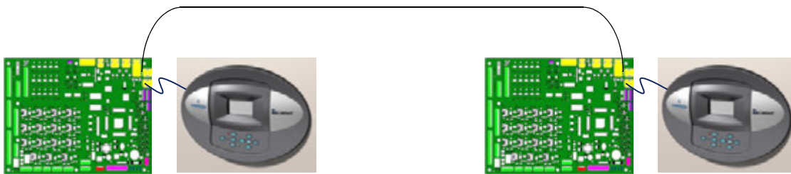
Figure 77 Connecting two cooling units, each with a small display, using a crossover Ethernet cable
