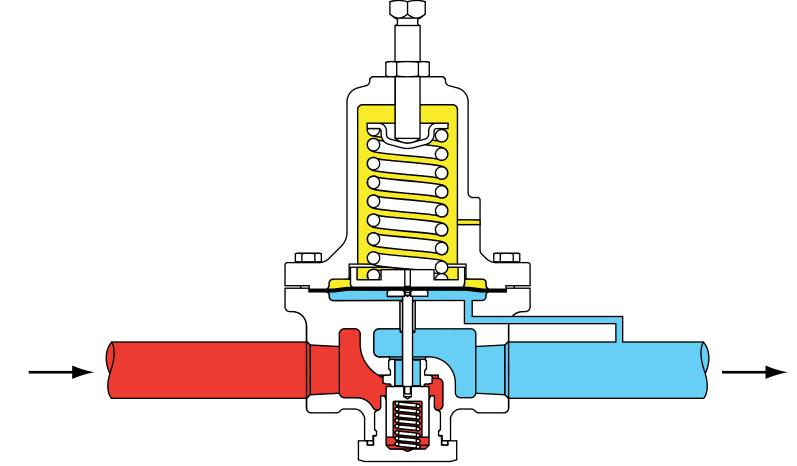
INLET PRESSURE OUTLET PRESSURE ATMOSPHERIC PRESSURE
