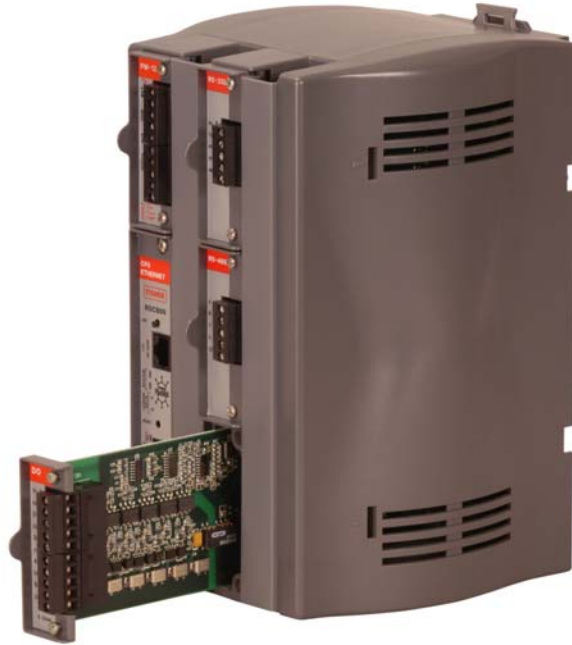
Figure 4-3. Installing an I/O Module
