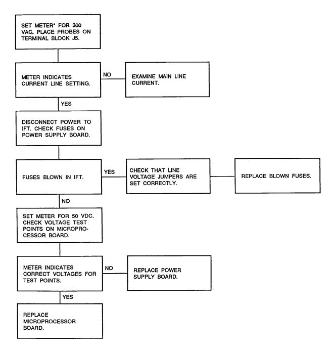
\*SIMPSON MODEL 260 OR EQUIVALENT MULTIMETER.
