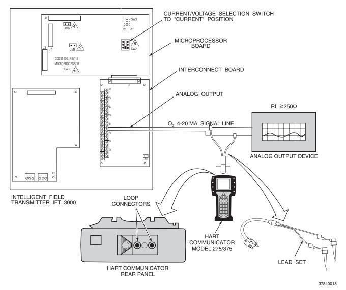
Figure J-2. Signal Line Connections, > 250 Ohms Load Resistance
