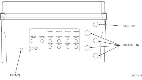
Figure 2-18. MPS Gas Connections
