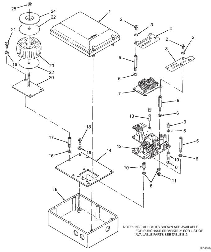
Figure B-7. Heater Power Supply, Exploded View
