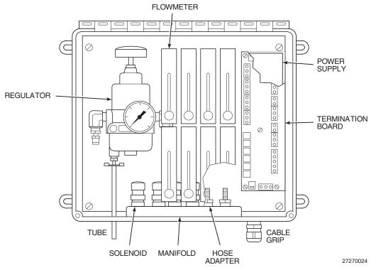
Figure D-2. Multiprobe Calibration Gas Sequencer, Interior
