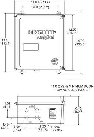
NOTE: DESIGN DIMENSIONS ARE IN INCHES WITH MILLIMETERS IN PARENTHESES.
