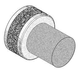
Figure A-13. Cup-Type Diffusion/Dust Seal Assembly
