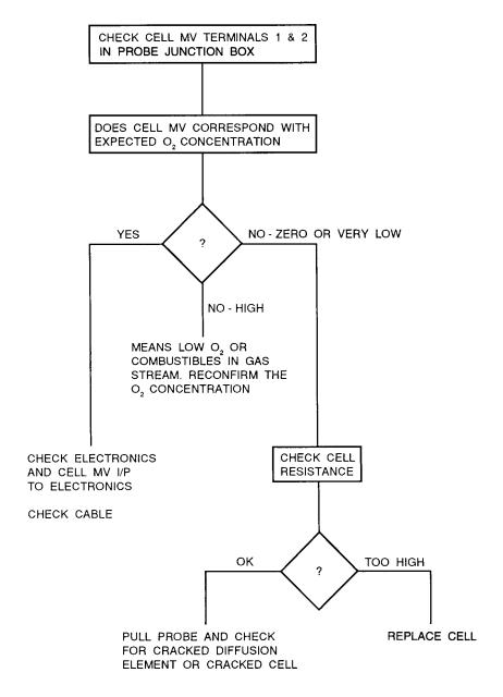
Figure A-16. Flowchart of Probe Related Problems, #1
