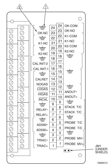
Figure 2-11. IFT Interconnect Board Output Connections
