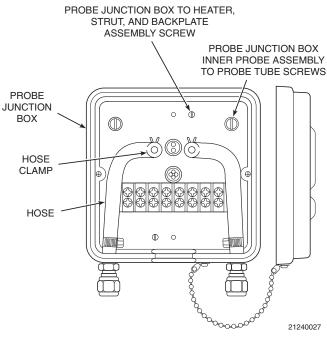
Figure A-21. Probe Junction Box Mechanical Connections
