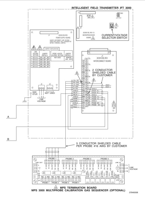
Figure 2-13. Wiring Layout for Complete IFT 3000 System with HPS (Sheet 2 of 2)
