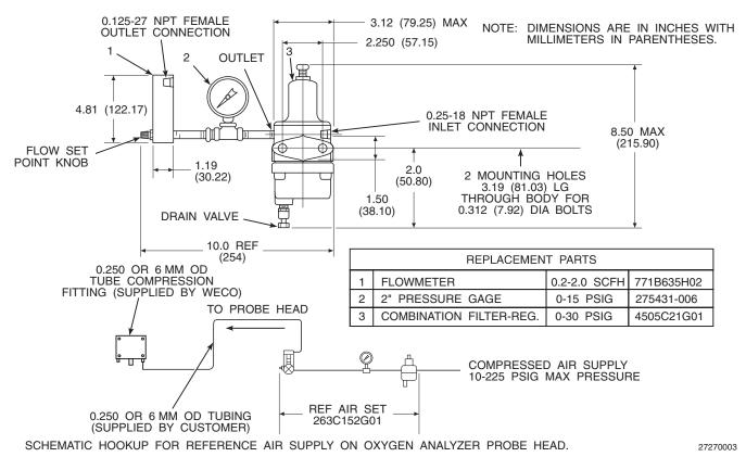
Figure 2-3. Air Set, Plant Air Connection
