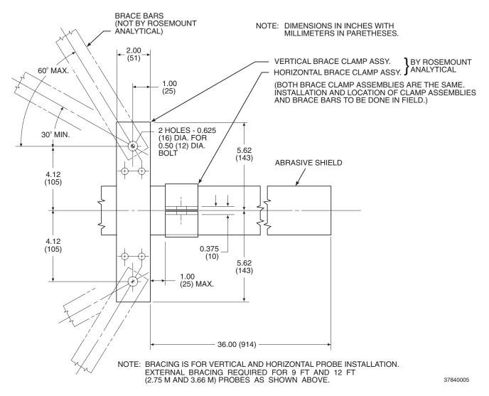
Figure 2-1. Probe Installation (Sheet 5 of 5)
