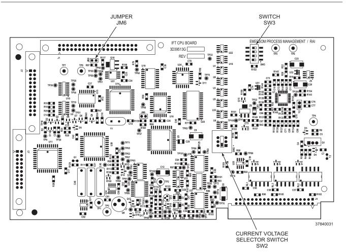
Figure 2-9. IFT Microprocessor Board
