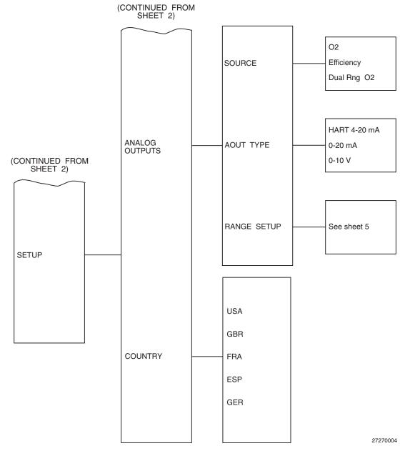
Figure 5-2. Quick Reference Chart (Sheet 3 of 5)
