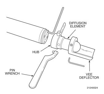
Figure A-4. Optional Ceramic Diffusor and Vee Deflector Assembly
