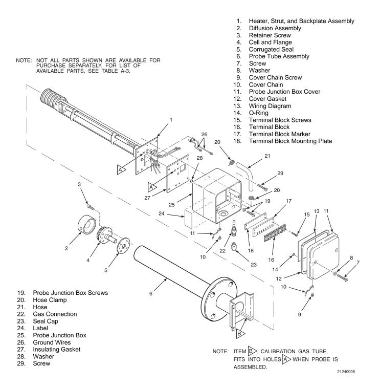
Figure A-1. Oxygen Analyzer (Probe) Exploded View
