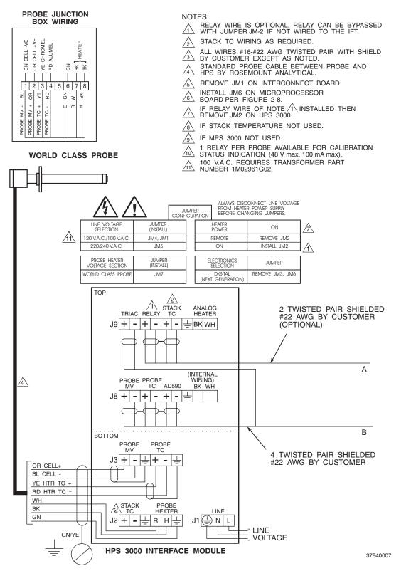
Figure 2-13. Wiring Layout for Complete IFT 3000 System with HPS (Sheet 1 of 2)
