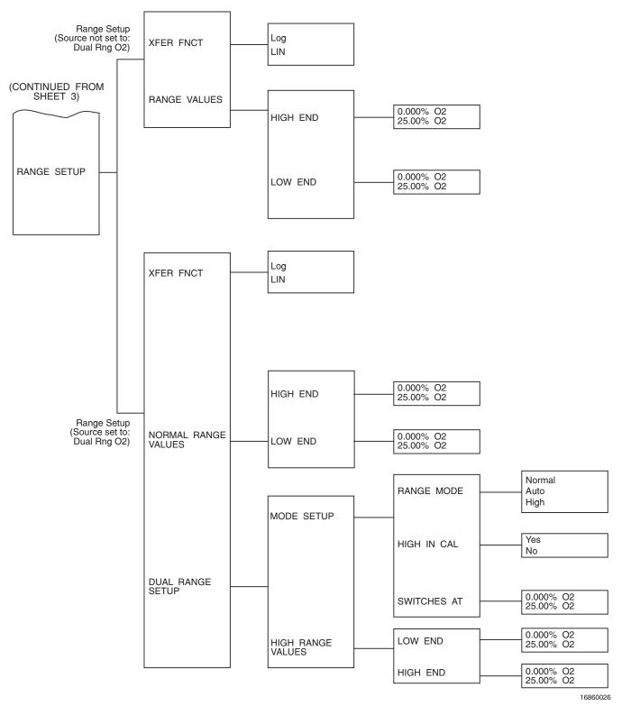
Figure 5-2. Quick Reference Chart (Sheet 5 of 5)
