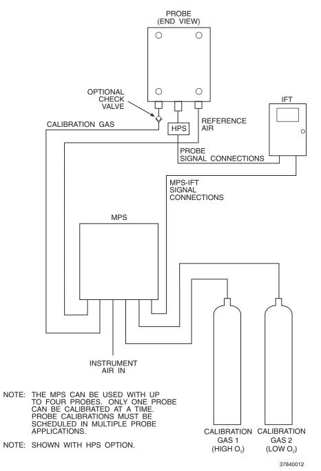
Figure D-3. Typical Automatic Calibration System
