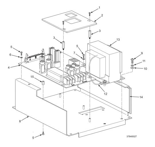
Figure E-8. Electronics Chassis – Exploded View
