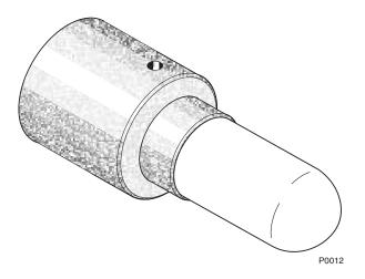
Figure A-11. Flame Arrestor Diffusion Assembly
