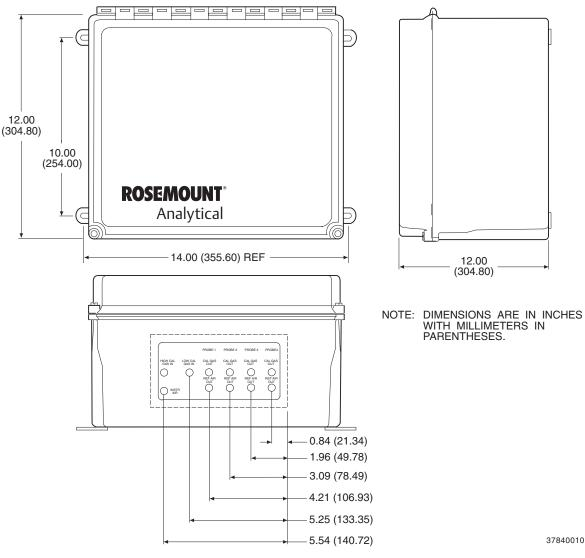
Figure 2-17. MPS Module
