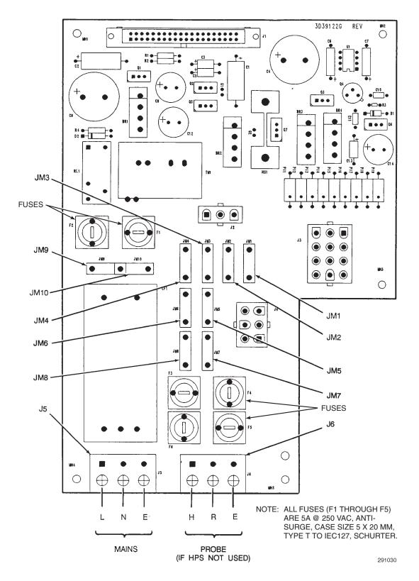
Figure 2-6. IFT Power Supply Board Jumpers
