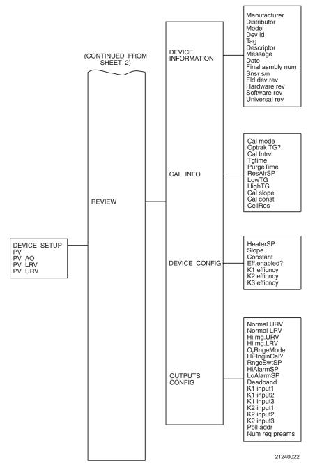
Figure J-4. Menu Tree for IFT 3000 Applications (Sheet 3 of 3)
