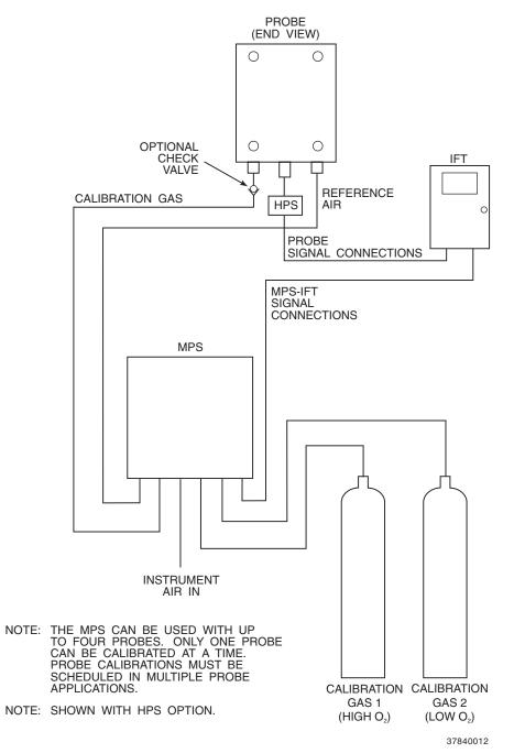
Figure 4-4. Typical Automatic Calibration System
