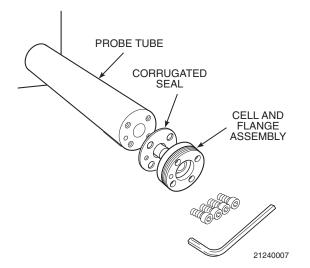
Figure A-3. Cell and Tube Assemblies
