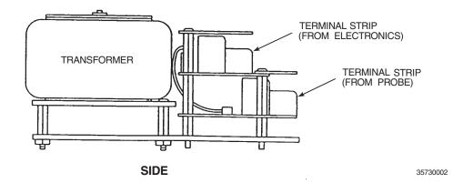
Figure B-2. Heater Power Supply, Interior
