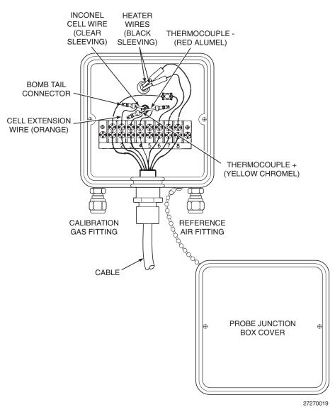
Figure A-18. Cell Wiring Connection
