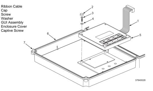
Figure E-10. Replacing the GUI Assembly
