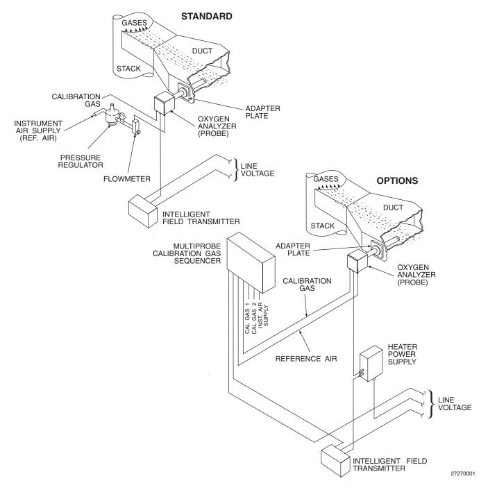
Figure 1-2. Typical System Installation
