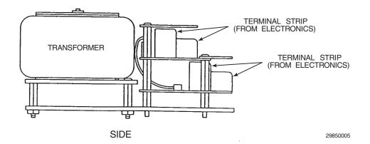
Figure 2-14. Heater Power Supply Wiring Connections
