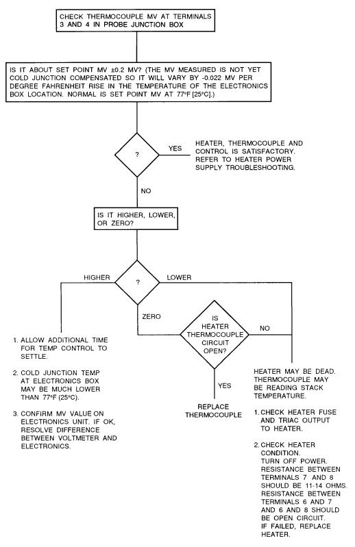
Figure A-17. Flowchart of Probe Related Problems, #2
