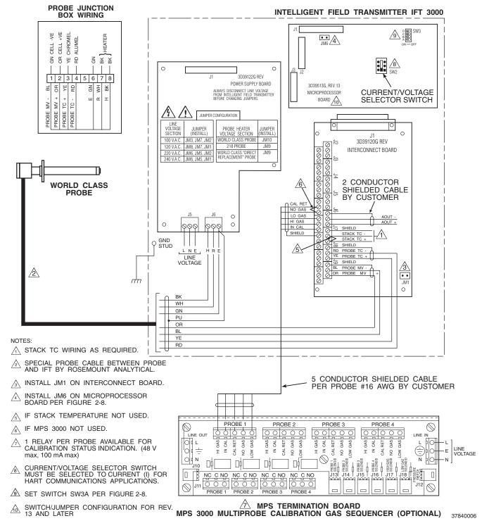
Figure 2-7. Wiring Layout for IFT Systems without HPS
