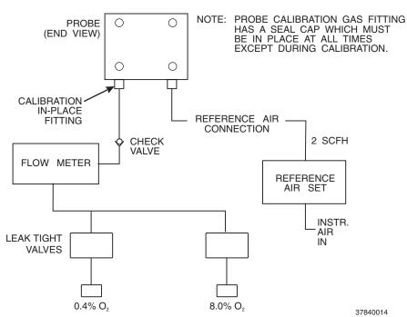
Figure 4-1. Typical Calibration Setup
