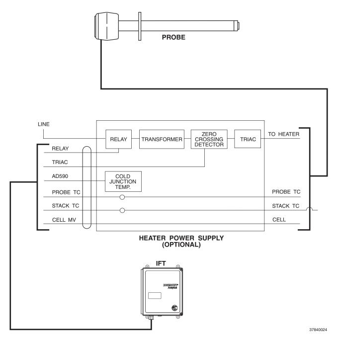
Figure E-2. System Block Diagram
