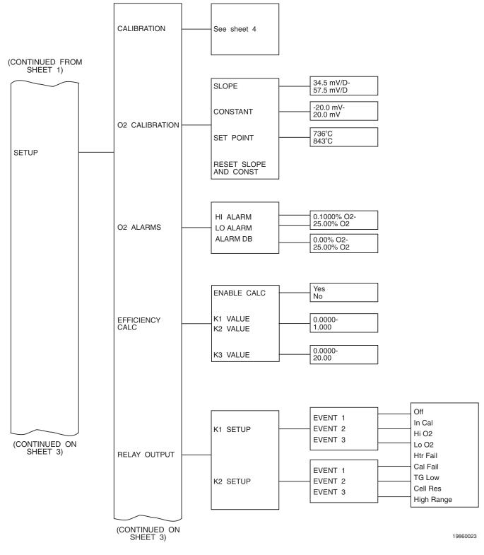
Figure 5-2. Quick Reference Chart (Sheet 2 of 5)
