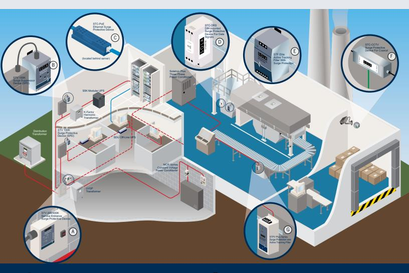
A **STV200/400K:** Surge protective devices capable of handling the high-impulse, potentially damaging transients commonly found at the service entrance, distribution panels, and placement in the most severe exposure locations.
