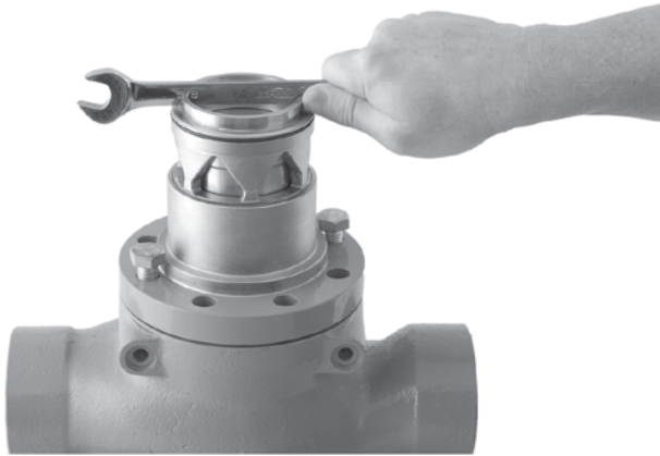
Figure 5. Seat Ring/Cage Removal or Installation Using Body as Holding Fixture
