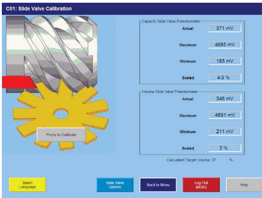
Figure 4-4. Slide Valve Calibration Screen (Compact Logix PLC)
