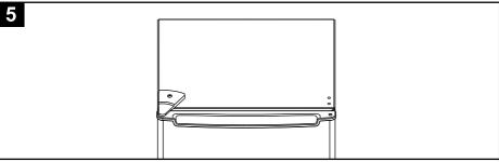
Check that the door is aligned horizontally and vertically and that the seals are closed on all sides before finally tightening the upper hinge. Re-adjust the leveling feet.
