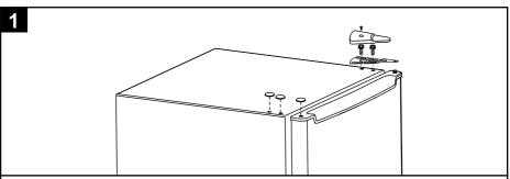
Unscrew the screw of top hinge cover, Remove the upper hinge cover, then unscrew the upper screws of metal hinge bracket and take off the hinge. Then take off the left side screw covers. Pull the appliance door upward to take it off.
