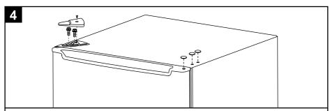
Slot the appliance door into the bottom hinge pin. Replace the upper hinge bracket on the new side and check the fitting between the door/ hinge moving smoothly. Then tighten the screws of the upper hinge bracket Replace the hinge cover and the right side screw covers, tighten the screw of top hinge cover.
