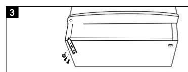
Install the leveling foot and the bottom hinge bracket on the new bottom side. Then tighten the screws of the bottom hinge bracket.
