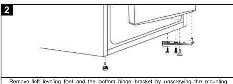
Remove left leveling foot and the bottom hinge bracket by unscrewing the mounting screws.
