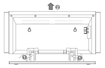
2.) Pull the main unit upward in the direction of the "arrow" to completely remove it.
