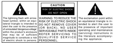
The Caution Marking was located at the rear enclosure of the apparatus.
