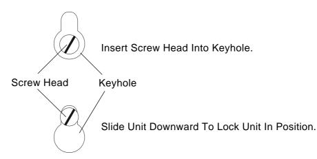
If the main unit is still loose, you probably left too large a gap between the screw head and the wall. Slide the unit slightly upward and take it off the mounting screws. Tighten one or both screws slightly and remount the unit. It should fit snugly against the wall and not move when you are loading or unloading CD's.
