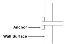
8.) Insert the screw into the anchor and tighten the screw until it touches the collar on the anchor. This causes the anchor to spread inside the wall and locks the anchor in place.
