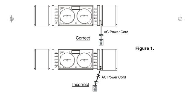
Connect the main unit to the AC outlet and position it against the wall in your desired location. Make sure that the plug remains firmly and full inserted into the outlet. There should be just enough slack in the power cord so that the plug can be easily removed from, and reconnected to the AC outlet.
