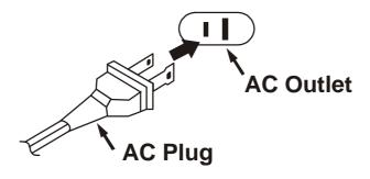
**Note:** Be sure to connect this radio to an outlet that is always 'live'. Do not connect this unit to an outlet that is controlled by a wall switch.
