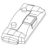
2.) Position the pedestal base so that the 4 guide hooks on the base slide into the 4 slots on the back of the main unit.
