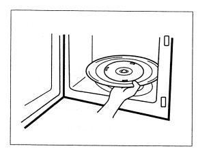
The roller guide and oven cavity floor should be cleaned regularly to avoid excessive noise.
