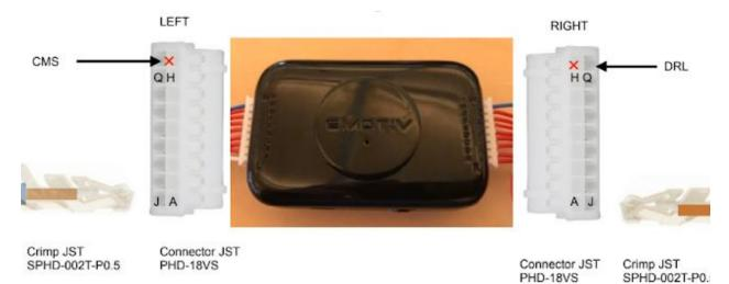
The EPOC Flex controller pictured above has 16 channels connected on the left + CMS input and 16 channels on the right + DRL output. These channels are connected in two rows A-H and J-Q, In software L or R is added in front to make it LA, LB, etc and RA, RB, etc. These labels allow users to easily trace signal problems from the name shown on software to the sensor. The connectors shown are JST PHD-18VS which are easily sourced from digikey if replacements are required.
