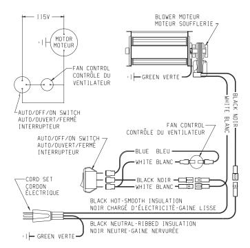
IF ANY OF THE ORIGINAL WIRE AS SUPPLIED WITH THIS UNIT MUST BE REPLACED. IT MUST BE REPLACED WITH NO. 18, 150  $^\circ\mathrm{C}$  WIRE OR ITS EQUIVALENT.
