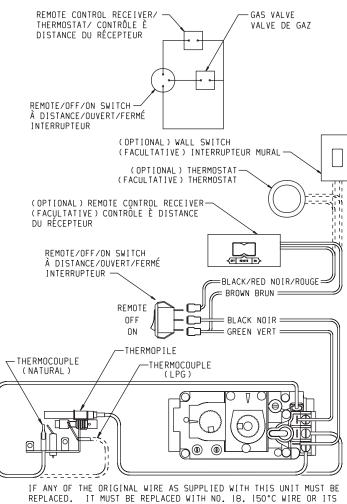
REPLACED. IT MUST BE REPLACED WITH NO. 18, 150°C WIRE OR EQUIVALENT. Figure 21
