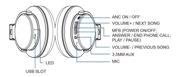
Power On: Press center key for 3 seconds Power Off: Press center key for 3 seconds
